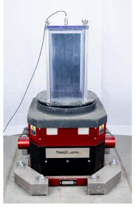
CB elimination device for basic research: Verification of the theory of eliminating CB (Concrete Bubble) generated during concrete placing, discovering new correlations and laws, extract optimal variable inertia force conditions for each blending composition.
