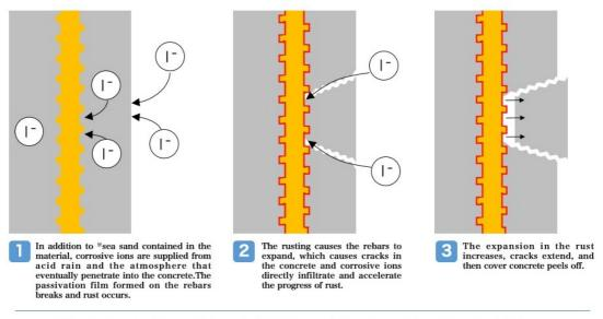
\*\* In addition to using sea sand as a material, corrosive ions are also supplied from the atmosphere, exhaust gas, acid rain, etc., which penetrate into the concrete and rust occurs due to defects in the passivation film of the rebars.
